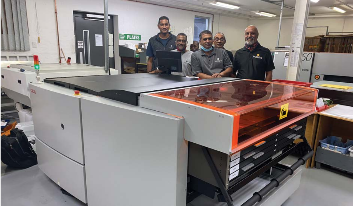
The Cron UVP-4648G+ computer-to-plate system can process and punch lithographic printing plates with minimum dimensions of 280 x 280mm and maximum dimensions of 1 160 x 960mm and that vary in thickness from 0.13 to 0.4mm.
